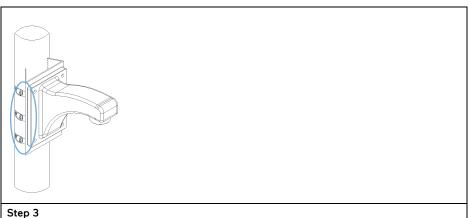
Fasten straps securely with flathead screwdriver
