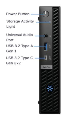
**Front Panel Connections & Controls**
