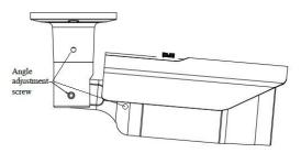
Figure 2-4 Adjust the camera angle
