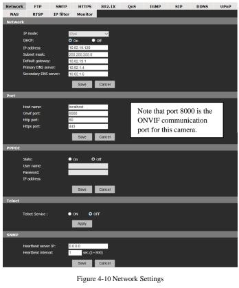
There are 14 option tabs for settings: Network, FTP, SMTP, HTTPS, 802.1X, QOS, IGMP, SIP, DDNS, UPnP, NAS, RTSP, IP Filter and Monitor.
