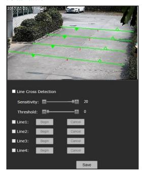
Figure 4-50 Line Cross Detection
