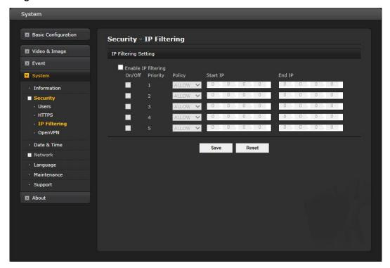
Checking the "Enable IP address filtering" box enables the IP address filtering function. When the IP address filter is enabled, addresses added to the list are set as allowed or denied addresses. All other IP addresses not in this list will then be allowed or denied access accordingly, that is, if the addresses in the list are allowed, then all others are denied access, and vice versa.
