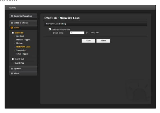
This is used to trigger the event every time the network connection fails. Select "Enable network loss" to activate the Network Loss event. Select a dwell time for how long the event will last from the point of detection.
