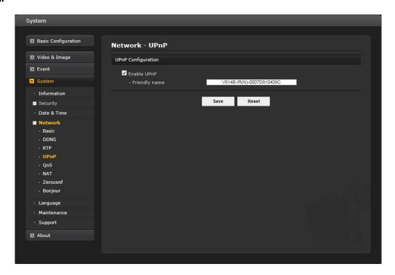
The network camera includes support for  $UPnP^{TM}$ . UPnP is enabled by default, so the network camera is automatically detected by operating systems and clients that support this protocol. Enter a name in the Friendly name field.
