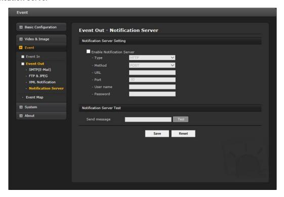
When the network camera detects an event, the Notification Server is used to receive uploaded image files and/or notification messages. Check the box to enable the service.
