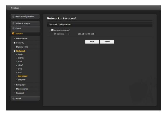
Zero configuration networking (zeroconf) is a set of techniques that automatically creates a usable Internet Protocol (IP) network without manual operator intervention or special configuration servers.
