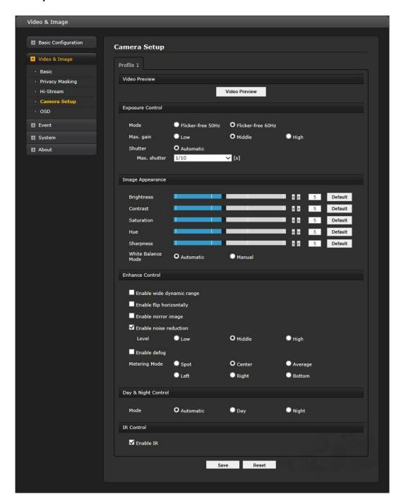
From this page, user can setup Exposure Control, White Balance Control, Image Appearance, and Day & Night control.
