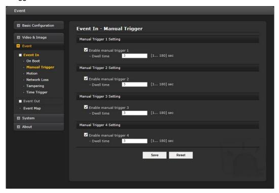
This option makes use of the manual trigger button provided on the Live View page, which is used to start or stop the event type manually. Alternatively, the event can be triggered via the product's API (Application Programming Interface).
