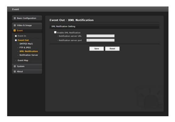
When the network camera detects an event, Notification server is used to receive notification messages as a type of XML data format. Check the box to enable the service.
