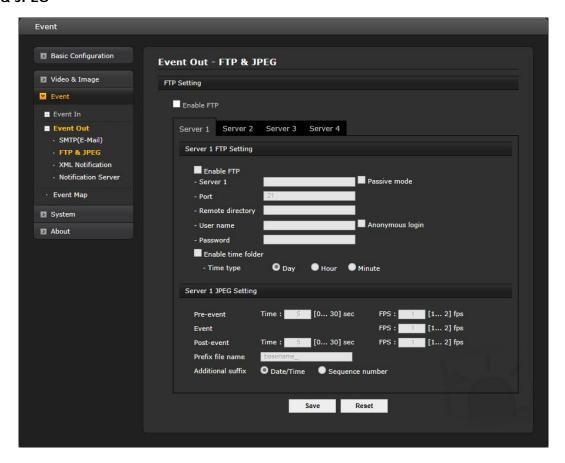
When the network camera detects an event, it can record and save images to an FTP server. Images can be sent as e-mail attachments. Check the "Enable FTP" box to enable the service. This camera can support multiple FTP servers and user can configure each server settings separately.
