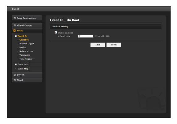
This is used to trigger the event every time the network camera is started. Select "Enable on boot" to activate the motion event.
