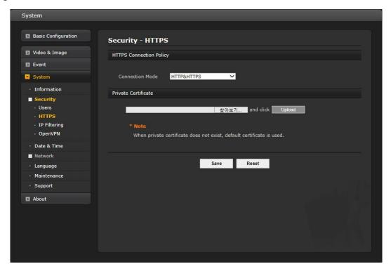
For greater security, the network camera can be configured to use HTTPS (Hypertext Transfer Protocol over SSL (Secure Socket Layer)), so that all communication that would otherwise go via HTTP will instead go via an encrypted HTTPS connection.
