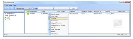
4) Select Assign IP. The Assign IP window displays. Enter the required IP address.
