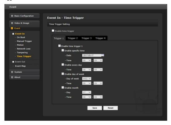
Time Trigger is to set alarms at specific time. User can set up to four (4) time triggers and each time trigger can be set to a specific date in the calendar, every day, day of the week, or date of every month.
