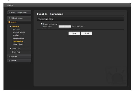
This is used to trigger an event when tampering with the camera occurs, for example, obstructing the camera with foreign material or moving the camera direction using external force. Select "Enable tampering" to activate the Tampering event.
