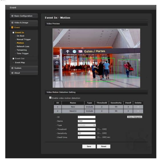
Motion detection is used to generate an alarm whenever movement occurs (or stops) in the video image. A total of 8 Motion and/or Mask windows can be created and configured.
