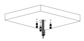
2. Pull the safety wire and cables through the bottom case of pendant mount and tighten the screws.
