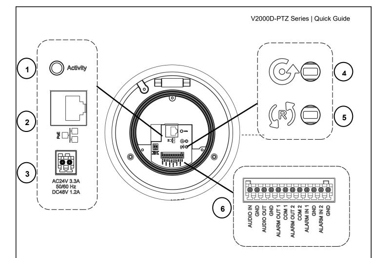
Figure 1 - 3: Internal Interface Pictorial Index
