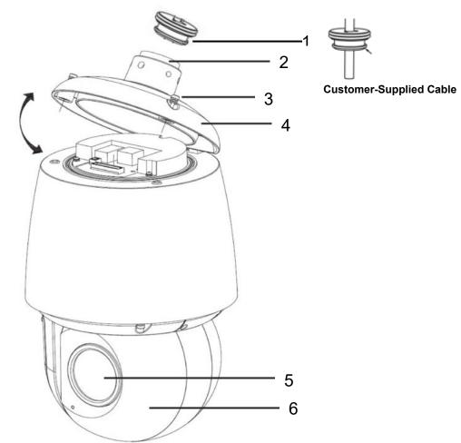
Figure 1 - 2: Parts Pictorial Index
