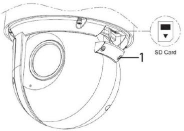
Figure 2 - 1: Inserting or Removing The Micro SD Card
