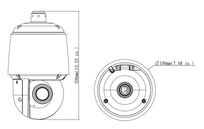
Figure 1 - 1: Physical Dimensions Unit: mm (in.)
