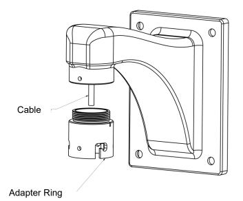
Figure 2 - 2: Locking the Pendant Adapter
