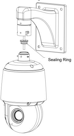
Figure 2 - 3: Mounting the Camera
