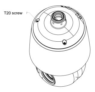
Figure 2 - 5: Loosening the 2 T20 Screws on Top Cover
