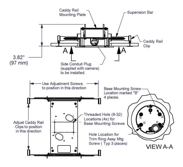
Figure 4 V2000D-ICD Installation
