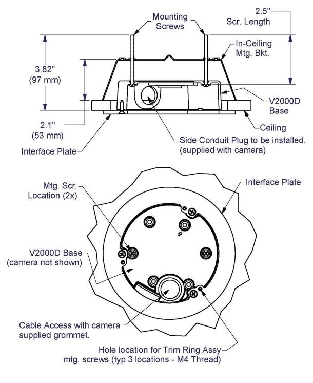
Figure 3 V2000D-ICH Installed Position
