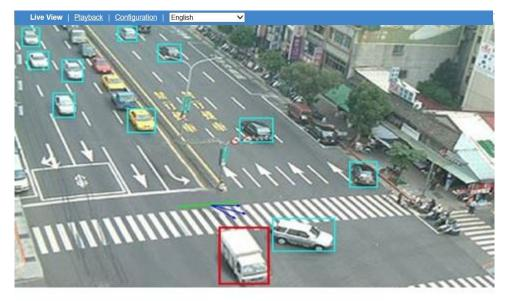
Figure: Wrong Direction Performance On Live View
