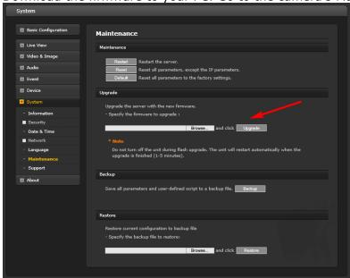
Open the Upgrade section and use the Browse button to locate the firmware on your PC. Press the upgrade button. During the upgrade process, do not turn off power to the camera. Wait at least 5 minutes and access the camera again. Once complete, the firmware version can be checked from the Basic Configuration screen.
