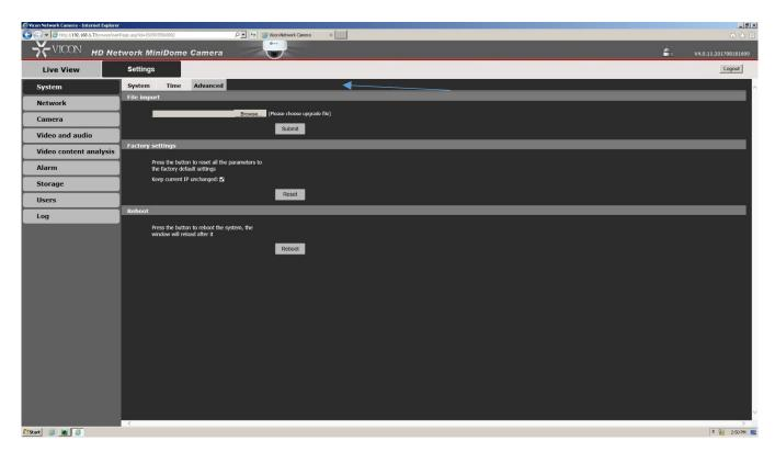
When the camera reboots the updated firmware will be installed. This can be checked by verifying the firmware version loaded in the upper right corner of the **Settings** page.
