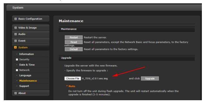
Open the Upgrade section and use the Browse button to locate the firmware on your PC. Press the upgrade button. During the upgrade process, do not turn off power to the camera. Wait at least 5 minutes and access the camera again.
