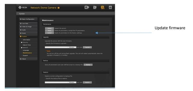
Open the Upgrade section and use the Browse button to locate the firmware on your PC. Press the upgrade button. During the upgrade process, do not turn off power to the camera. Wait at least
