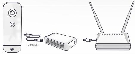
Connect to your door hardware (e.g., electronic locks, door contacts, etc.) and plug reader into a PoE switch to power it up. Connect the PoE switch to your router so you can access your reader via the cloud.
