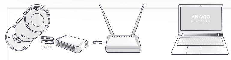
Install your camera and plug it into a PoE switch to power it up.
